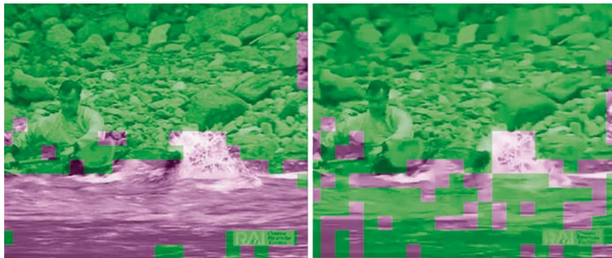
Fig. 4.18 Mode distribution of frame 4 in Rafting sequence using the exhaustive RDO-MD for two different QP values: Left : QP=16 and Right : QP=38
